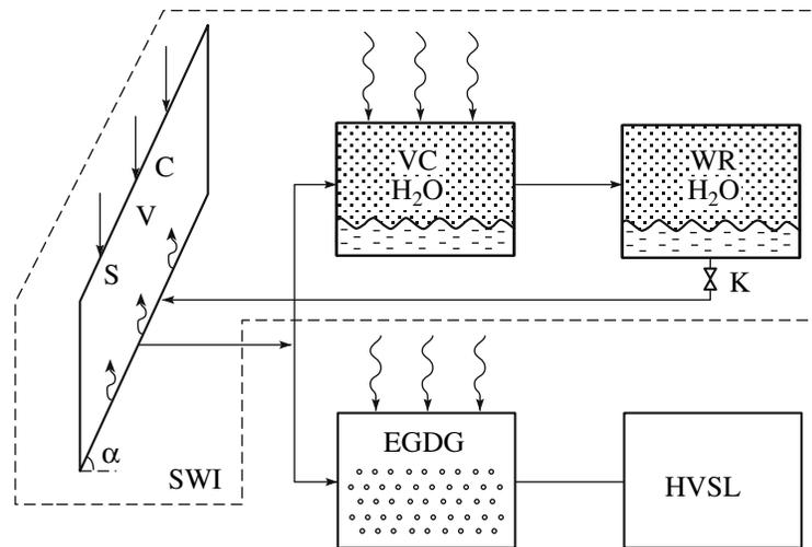
**Fig. 1.** Solar–wind energy complex. SVC is the solar vapor collector; VC is the vapor condenser; WR is the water reservoir; EGDG is the electrogasdynamic generator; HVSL is the high-voltage supply line; K is the faucet; ↓ is solar rays; ↷ is wind; ↑ is vapor.
